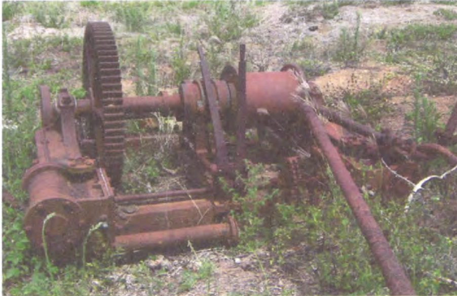
Figure 30 Walkers Ltd., Maryborough, Queensland, twin-cylinder steam winch (September 2010)
