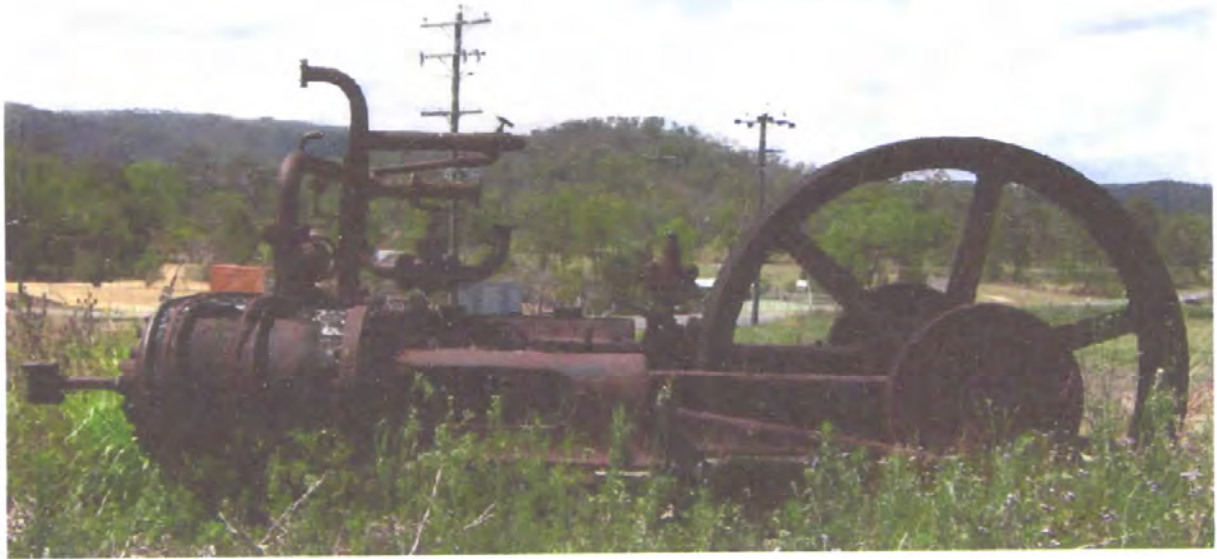
Figure 13 Marshall steam engine low pressure cylinder side. Note the tailrod crosshead guide at the left, and the bands on the cylinder body for retaining the wooden lagging (September 2010)
