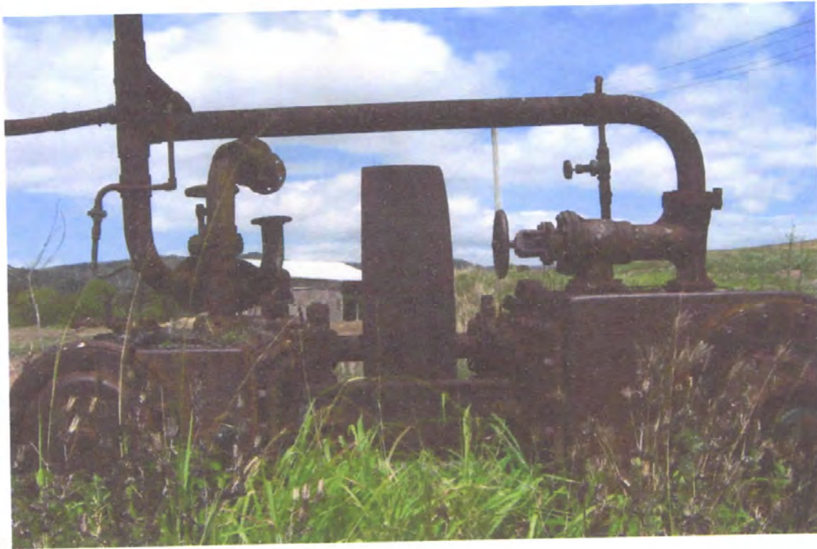
Figure 15 Marshall steam engine viewed from cylinder end, high pressure cylinder on the left, and low pressure cylinder on the right (September 2010)
